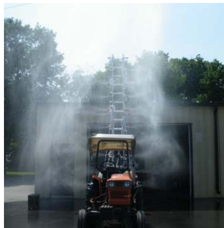
Test the sprayer plumbing and stability
